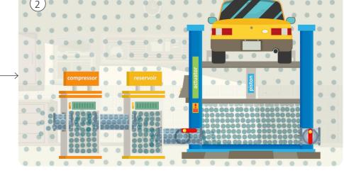
Air is sucked from the atmosphere and squashed in a compressor. The compressed air is stored under high pressure in a reservoir. When the in valve between the reservoir and the actuator is closed, air cannot move out of the reservoir and the piston remains down.
